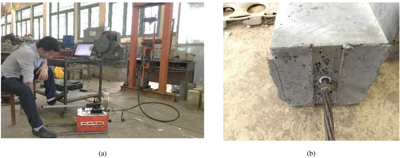
Fig. 3 - (a) The pull-out test in lab and (b) the specimen after testing
