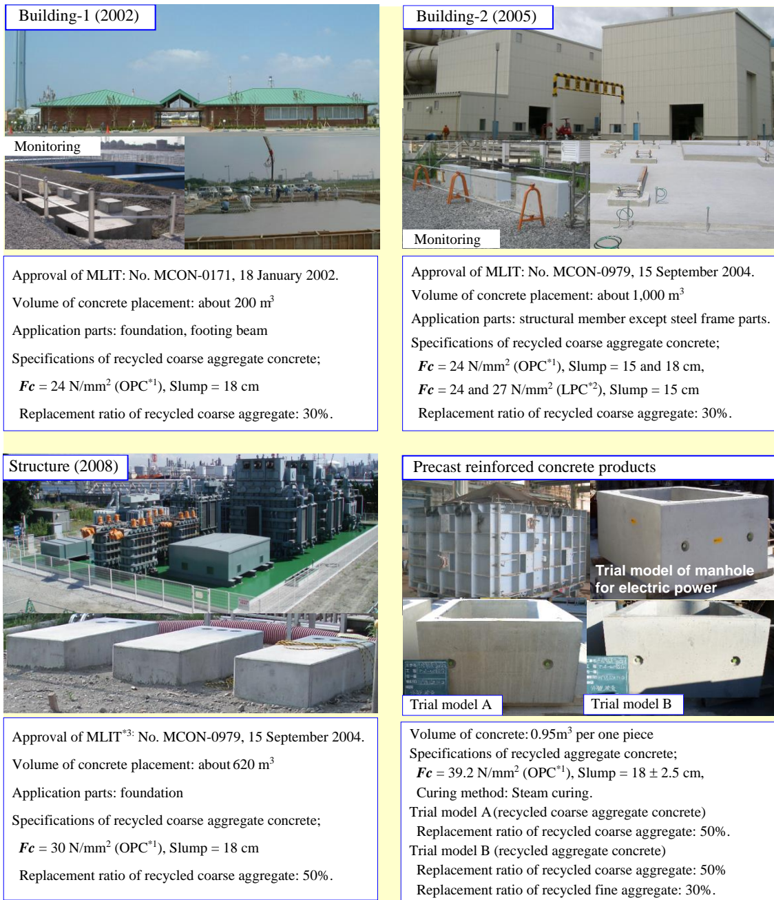
Fig. 2 – Appearance of recycled application examples of recycled aggregate concretes produced by the aggregate replacement method [8-11].
