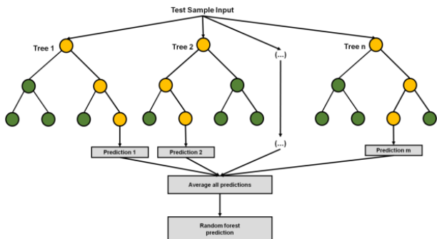
Figure 2. The RF prediction Algorithm
