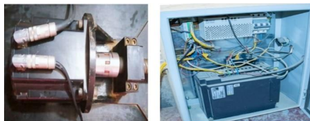
a. Servo motor b. Servo motor drive Plate 2. Servo motor and servo motor drive
