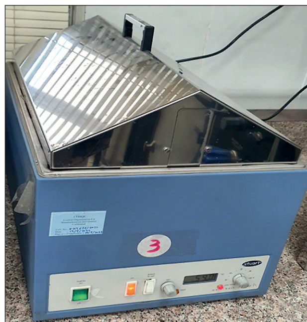
Fig. 2. Water path used in this research for curing samples at atmospheric pressure and heating temperature 60°C (140°F)
