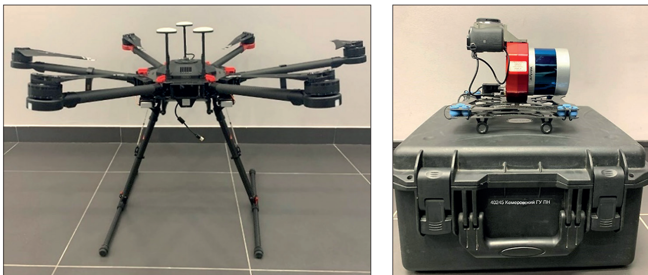
Fig. 1. General view of the equipment used in the study (on the left – UAV, on the right – an airborne laser scanner on a suspension)
