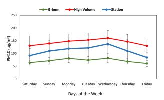
Figure 3. Daily variations of  $\mathsf{PM}_{_{10}}$  in TB monitor, high-volume sampler, and portable PM monitor
