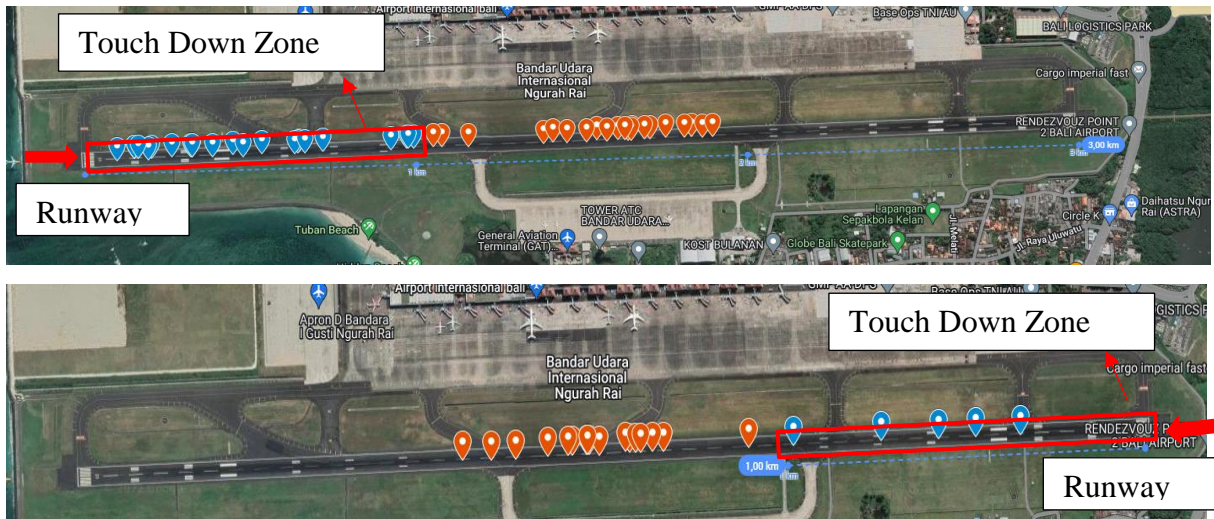
Fig. 7. Data points for the aircraft object landings at Denpasar Airport (DPS) runways 09 and 27
