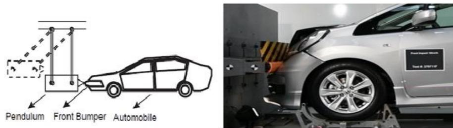
Fig. 25. Bumper impact test arrangement and image of the actual testing of a bumper
