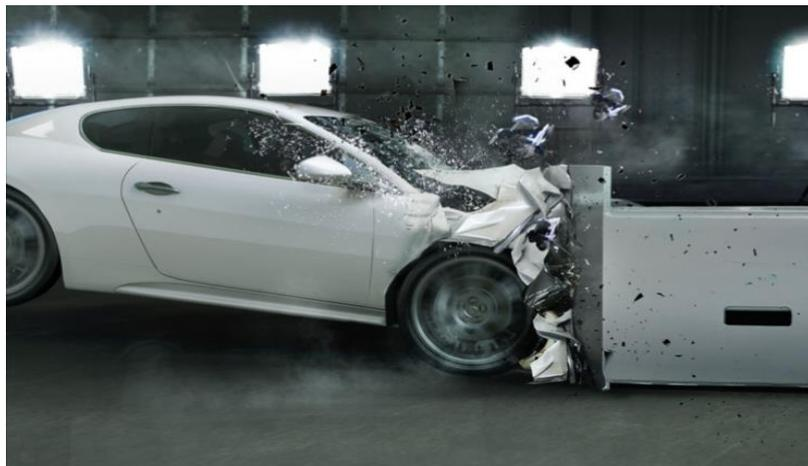
Fig. 23. Test image for a full-wrap frontal collision
