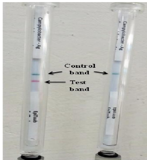
Figure 6. Campylobacter positive (colored test band) and negative samples by rapid immunochromatography test. Source: Gharst et al. (2013)
