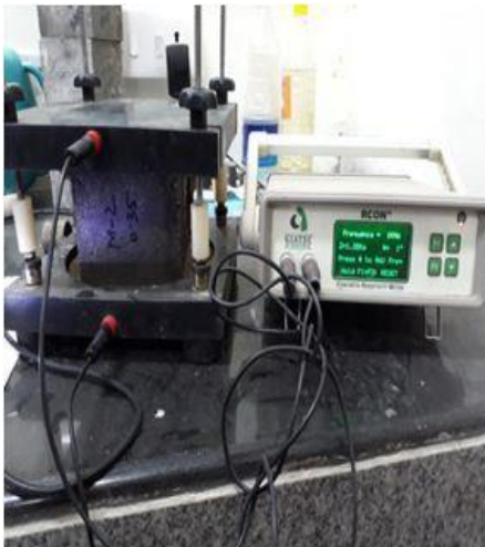
(a) ER equipment with concrete cube
