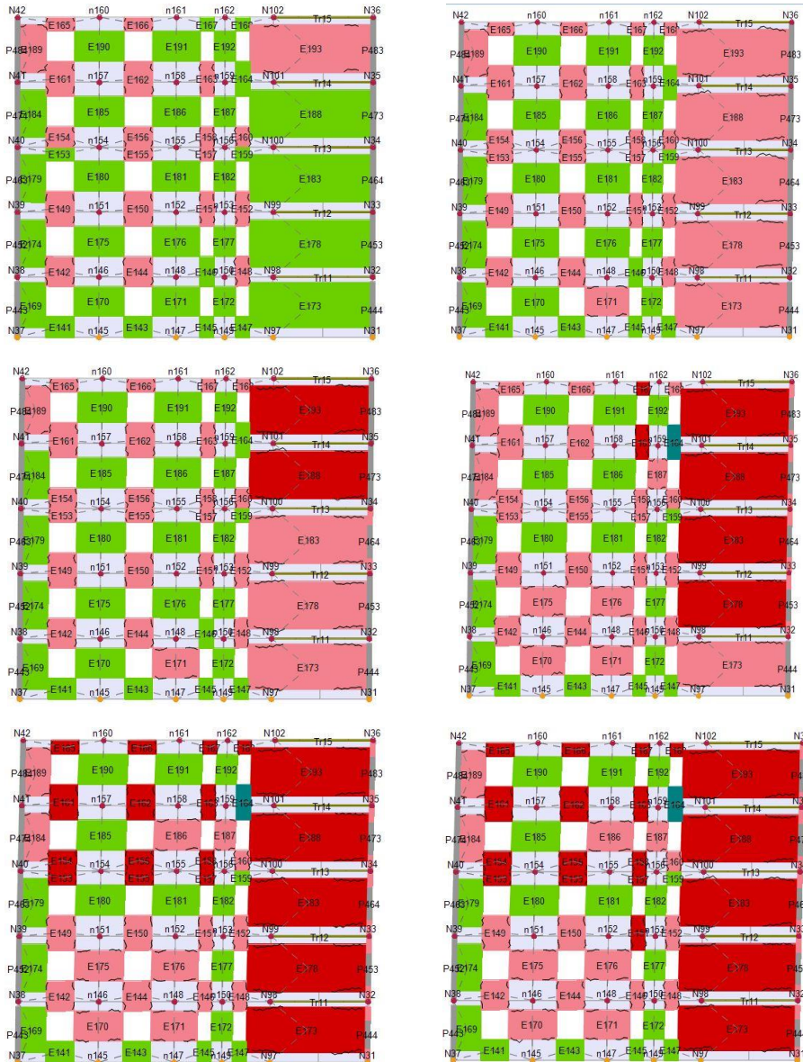
Fig. 21 Distribution of damage and the failure mechanism of perimeter walls from pushover analysis
