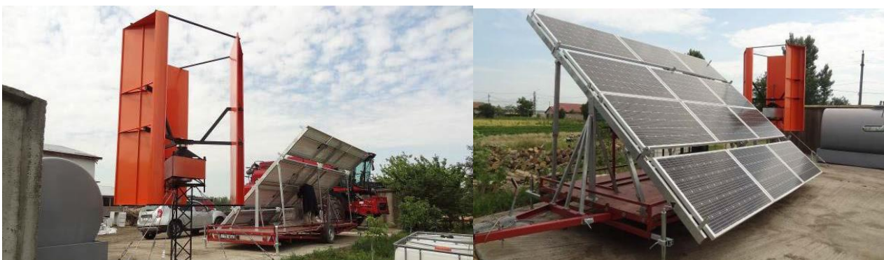
Fig. 2 - The mobile platform with wind turbines and solar panels for electric current production at agricultural farms in off-grid areas (Preda et al. , 2023).
