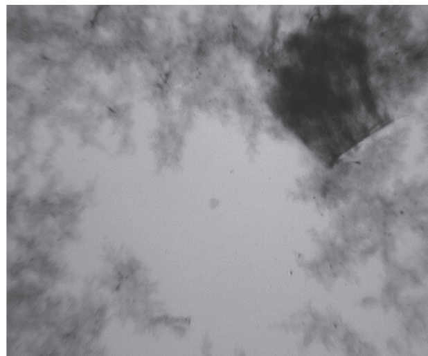
Fig. 1. Distribution of CNT in an aqueous dispersion of hyperplasticizer GP-60 (x5000)
