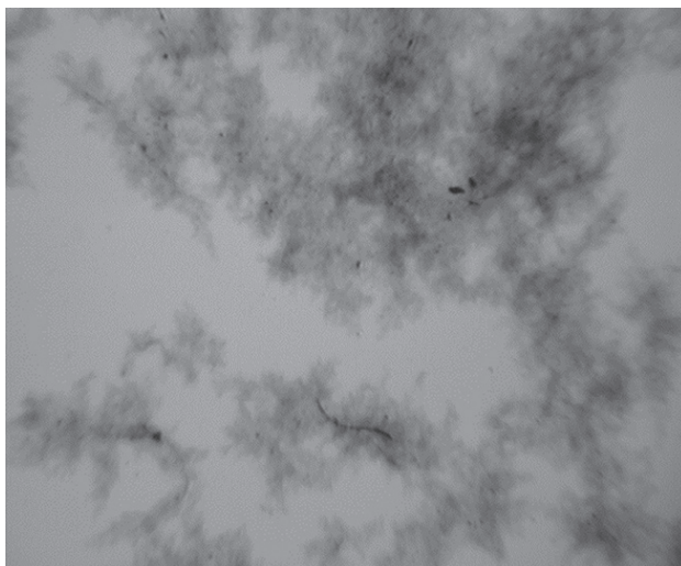
Fig. 1. Distribution of CNT in an aqueous dispersion of hyperplasticizer GP-60 (x5000)
