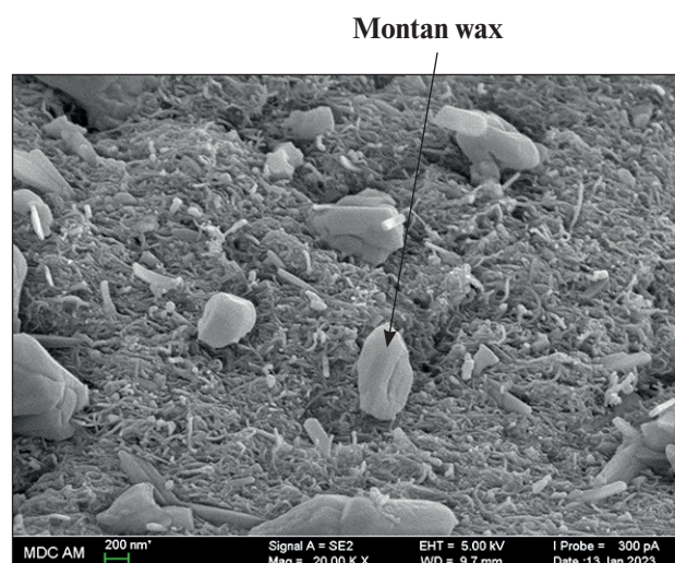
Fig. 1. SEM image of the surface of the CM-1230 complex modifier
