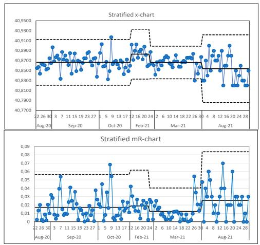
Figure 7. x-mR chart constructed by an expert
