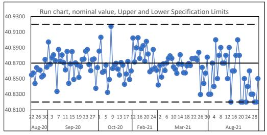
Figure 5. Run chart for the hole Ø40,87±0,05
