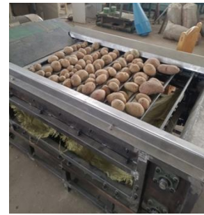
Fig. 6 - A full load of grading device
