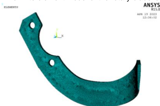
Fig. 3 – Finite element model of rotary blade
