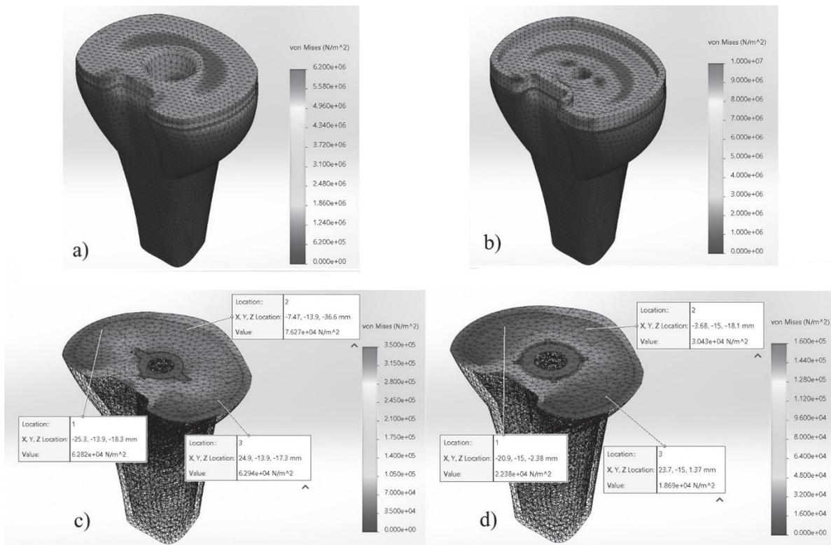
**Figure 3** Stress distribution when force of 1000N applied to 4-mm CoCr based tibial trays (a) and 2-mm Ti based tibial tray (b) simulated using SOLIDWORKS. Stress distribution on bone deep from surface 2 cm of Peripheral area of 2-mm Ti based tibial tray (c) and 4-mm CoCr based tibial tray (d)
