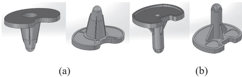
**Figure 2** Three-dimension model of the tibial tray developed in FE simulation (a) Cobalt chromium alloy with 4 mm -thickness (b) Titanium based alloy (Ti-6Al-4V alloy) and Cobalt chromium alloy with 2 mm-thickness
