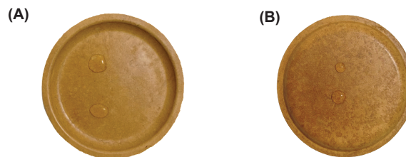
Fig. 8. Biodegradable trays based on RH and starch. (A) Frontside; (B) Backside.
