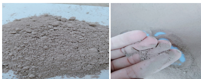
Fig. 1. Fly ash collected from the ESP system at Mong Duong 2 thermal power plant.
