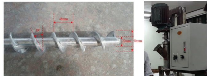
(A) Screw detail (used with permission from [14]) (B) Print-head system
