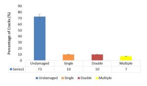
Fig. 5. Percentage of cracks in grains sample.
