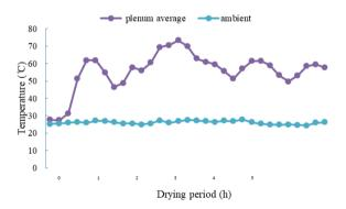
Fig. 3. Temperature variation at plenum and the ambient during the drying experiment.
