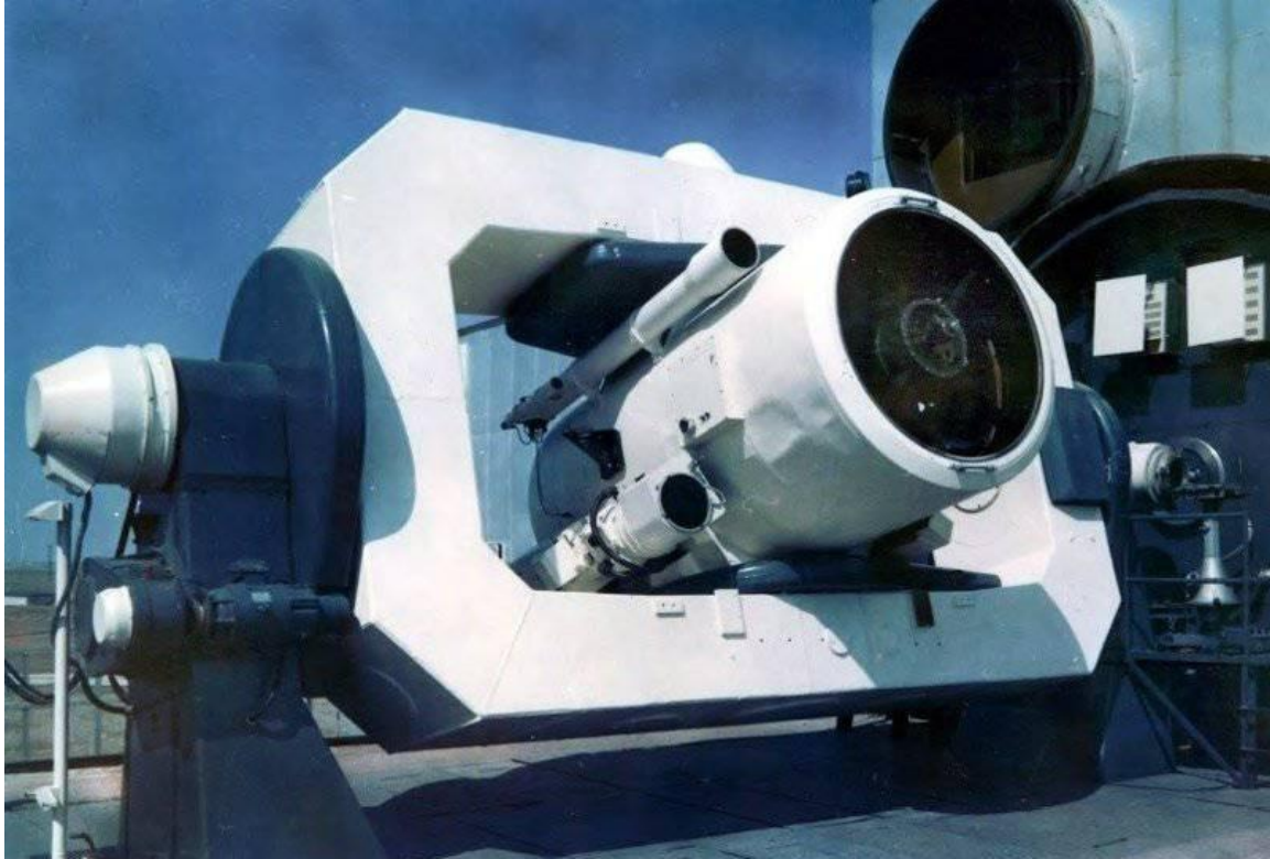
Figure 8. TG-1 telescope of the LE-1 laser locator, built for the “Terra-3” complex, Sary-Shagan test site (Zarubin & Pol’skikh, 2011).
