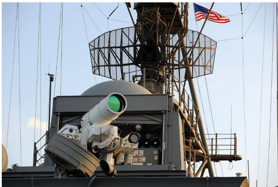
Figure 13. AN/SEQ-3 LaWS aboard USS Ponce (Zabunov & Mardirossian, 2020).
