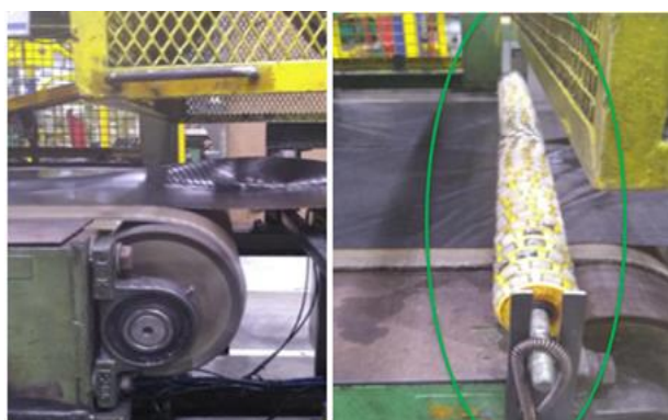
Figure 16. Before X After Inserting a roller on the take-up table (Source: Confidential).
