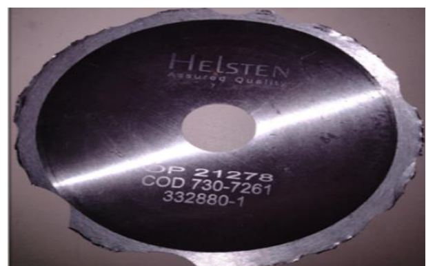
Figure 13. Knife Breakage due to entanglement (Source: Confidential)
