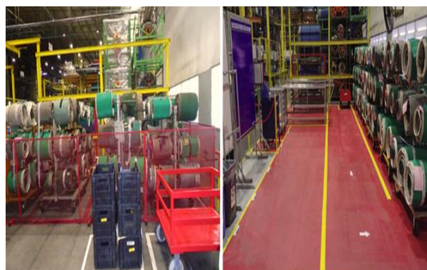
Figure 8. Before X After Flow creation for the input and output of NC material (FIFO) (Source: Confidential)
