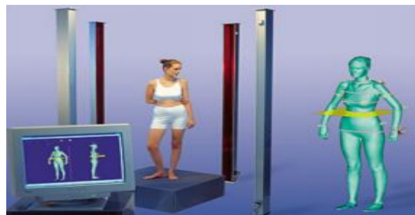
Figure 3. 3D body scanning by laser scanner
