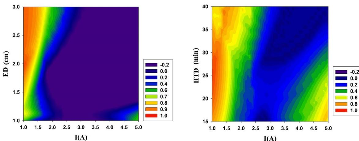
**Figure 4.** Response surface plots for overall desirability of GCS electrocoagulation using iron electrodes, for the variables ED (cm), I(A), and HRT (min).
