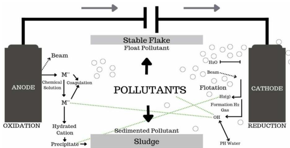
**Figure 1.** Schematic diagram of the electrocoagulation treatment.
