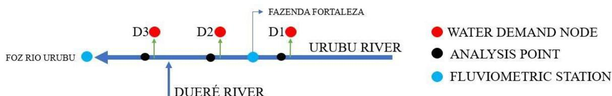
**Figure 7.** Single-line diagram of demand nodes and analysis points simulated in WEAP (Urubu River Basin/TO).
