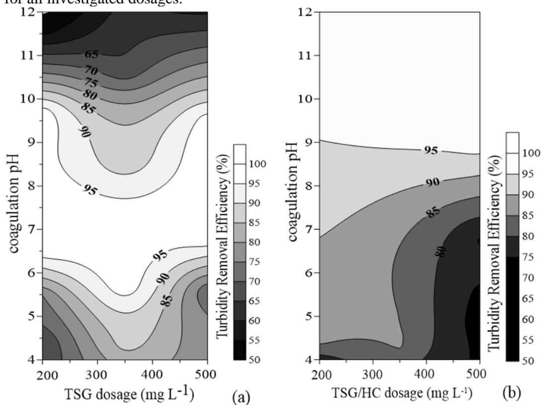
**Figure 2.** Coagulation diagrams for turbidity removal (%) from the industrial grain processing effluent using the coagulant: (a) TSG and (b) Tanfloc SG associated with Cationic Hemicellulose (TSG/CH 3:1 (v v<sup>-1</sup>)).
