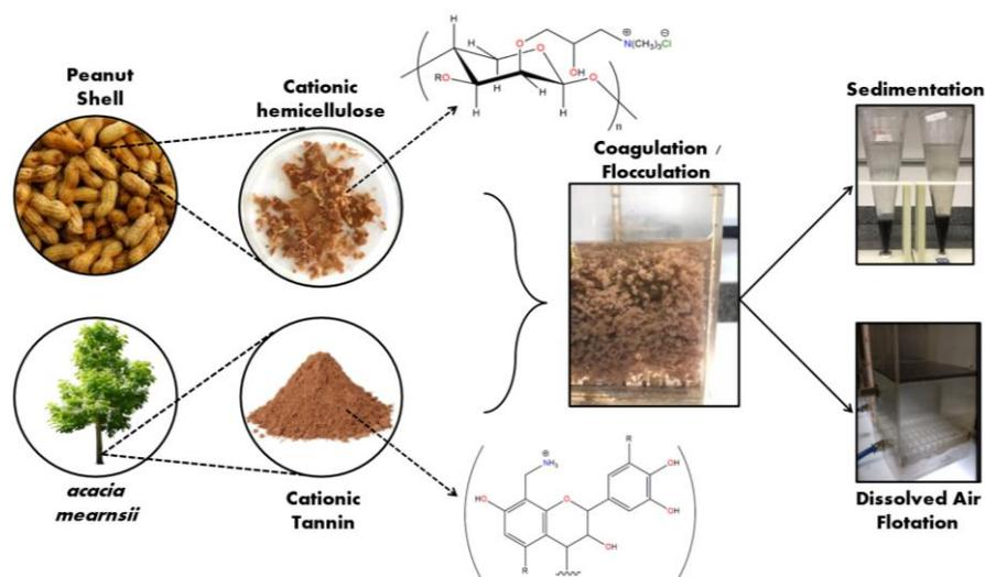
**Figure 1.** Schematic representation of coagulant synthesis from agro-industrial waste and effluent treatment.
