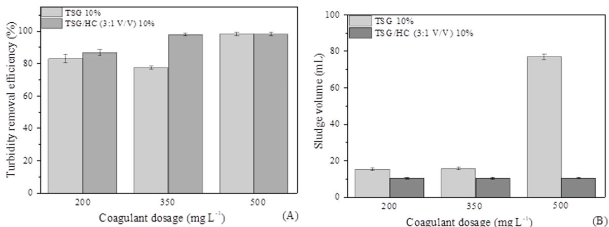
**Figure 4.** Turbidity removal efficiency (A) and Sludge volume formed (mL L<sup>-1</sup>) (B) for dissolved air flotation (DAF) applied after coagulation by TSG 10% and TSG/CH (3:1 v v<sup>-1</sup>) 10%.
