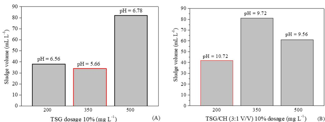
**Figure 3.** Sludge volume formation ( $\text{mL L}^{-1}$ ) after solid-liquid separation by physical-chemical treatment of the industrial effluent with sedimentation, for TSG and TSG/CH coagulants, respectively.
