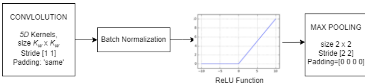
Figure. 8 Our proposed method: the fifth convolutional, batch normalization, ReLu, and max pooling
