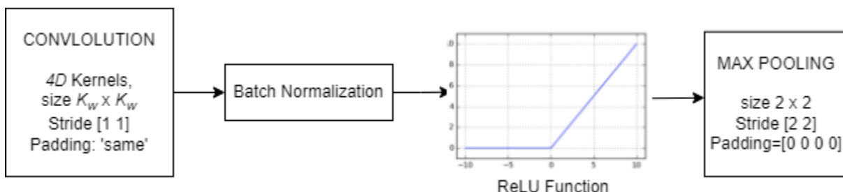
Figure. 7 Our proposed method: the fourth convolutional, batch normalization, ReLu, and max pooling
