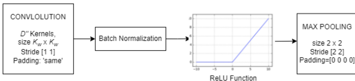
Figure. 4 Our proposed method: the first convolution, batch normalization, ReLu, and max pooling
