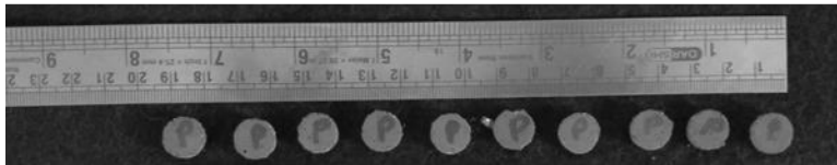
Fig. 1 Rocket Propellant Impregnated Brick Samples
