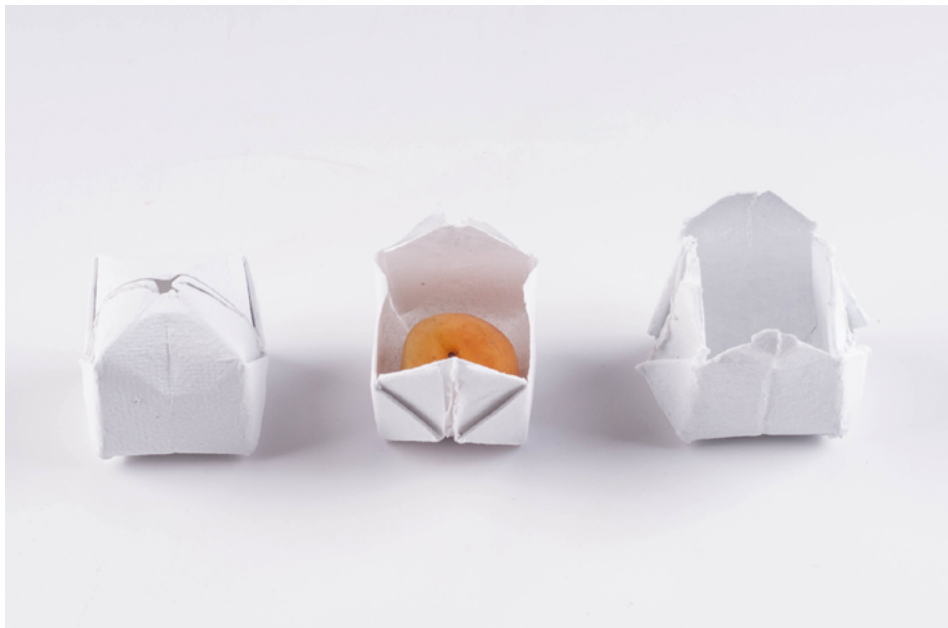
Figure 1. Mara Rossi, Dia_paper , experimental single-fruit packaging obtained by including diatomaceous earth powder in the cellulose, 2014. Coordination: Carla Langella.
