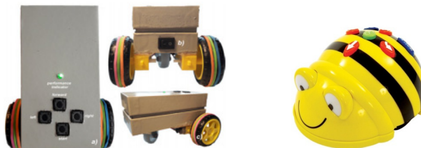
Fig. 2. Left: Robo-1 model: a) top view includes the control buttons and performance indicator; b) back view with the switch on-off button; c) general view of the robot; Right: Bee-Bot robot.
