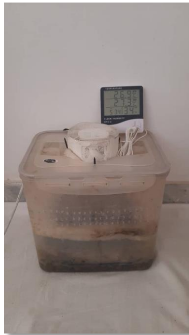
Fig. 8. Porous asphalt evaporation measuring device
