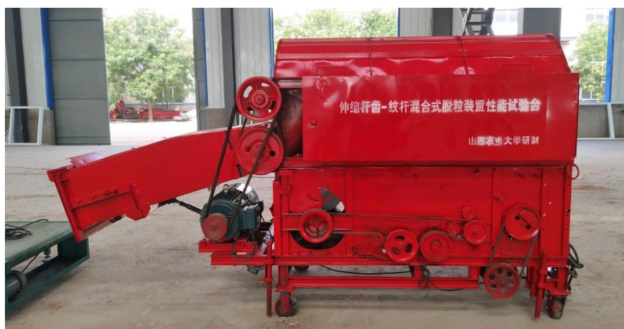
Fig. 5- Threshing device performance test bench
