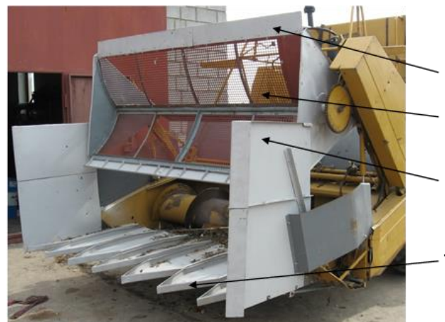
Fig. 6 - The design of the experimental header attachment of the "Sampo-500" plot combine for harvesting sunflower seeds
