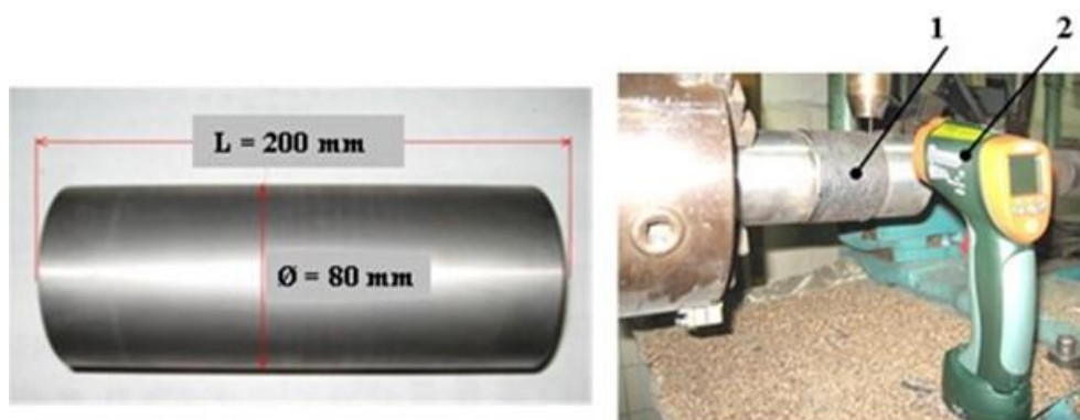
Fig. 1 - Cylindrical test specimen and process of weld deposition in a protective medium of carbon dioxide without vibrations of the welding wire 1 - specimen with deposited coating, 2 - infrared thermometer
