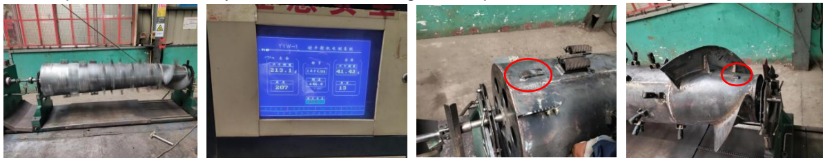
Fig. 6 - YYW-1 dynamic balancing machine and drum dynamic balance counter-weight results
