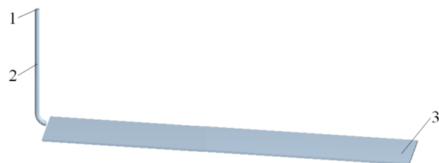
Fig. 6 - DEM simulation model 1 - particle factory; 2 – seed-guiding tube; 3 – soil
