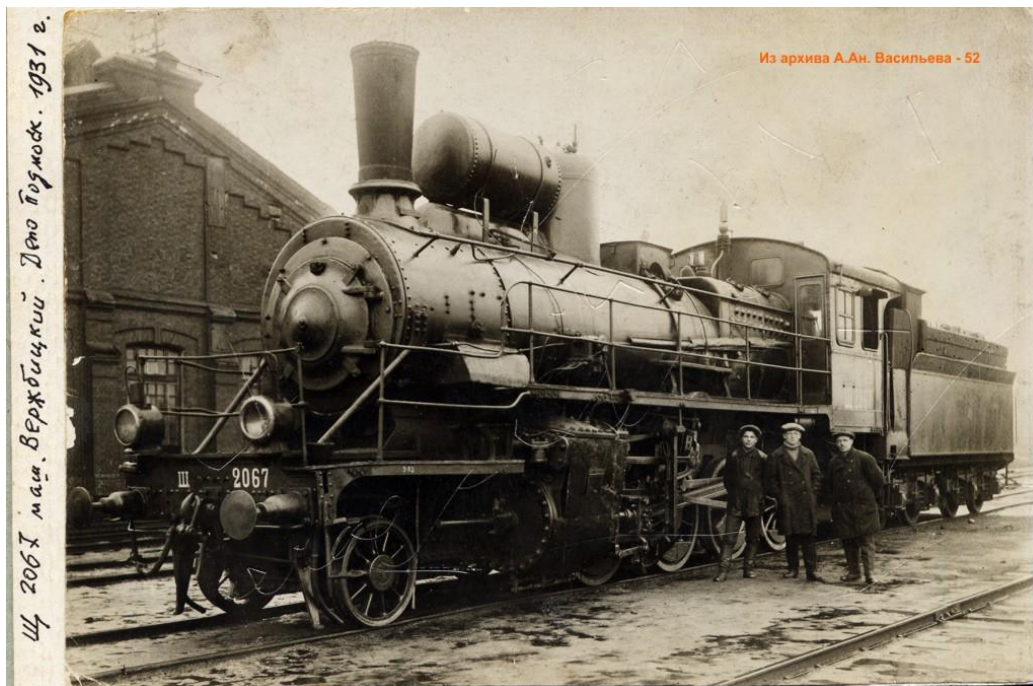
Figure 4. SHCH class steam locomotive. Steam locomotive series SHCH2067 (1931). Photo from the archive of A. A. Vasilyev-52. (TrainPix, 2017).
