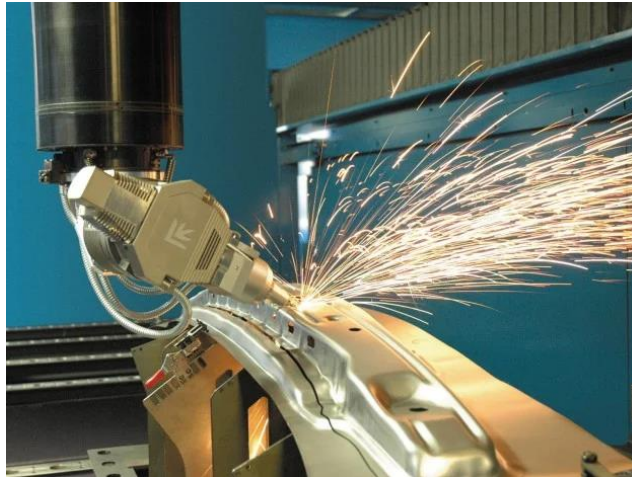
Figure 11. Three-dimensional laser cutting (3D fiber laser machine Rapido Prima Power).
