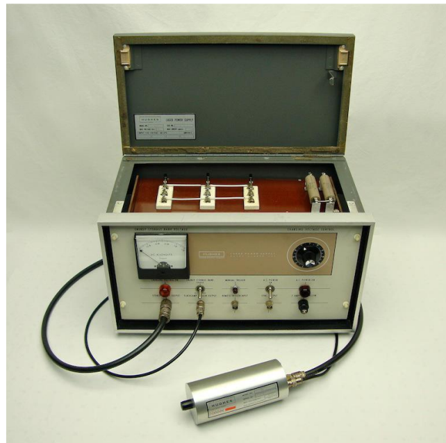
Figure 6. 1962 Hughes Aircraft Company model 200 ruby laser system, fully operational with all original components (Hess, 2013).
