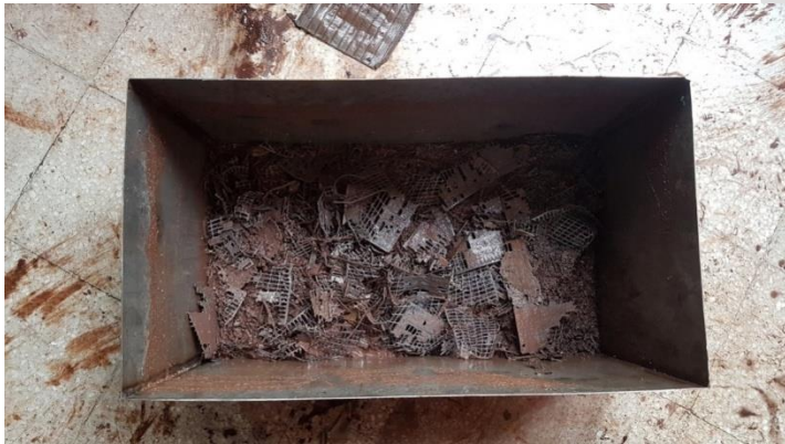
Figure 07: Sedimented lead along with some impurities and waste
