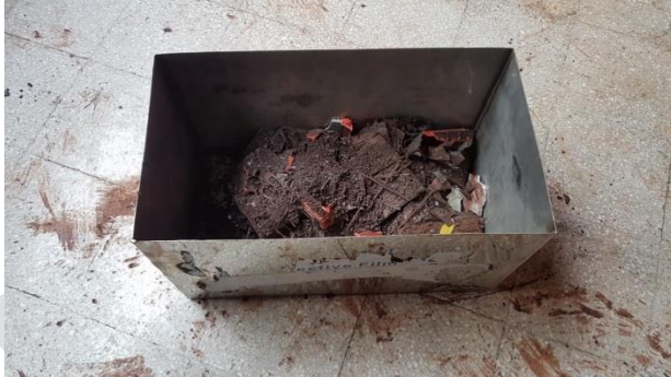
Figure 04: Crushed battery bits inside the hydro-separator
