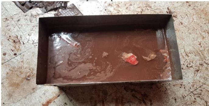
Figure 05: Hydro-separator filled with water and plastic bits floating up
