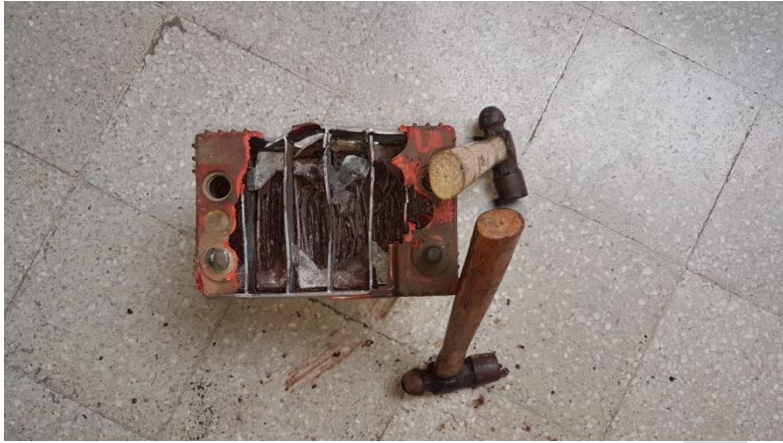
Figure 03: The battery being crushed using hammers
