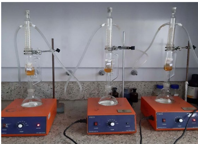
Figure 3: Soxhlet extractor for bioactive compounds extraction from S. marianum aerial parts
