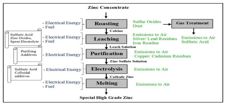
Figure 1: Hydrometallurgical process, energy consumption, and environmental aspects [18]
