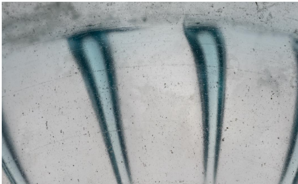
Fig. 10. Ribbed bowl (cat. no. 1): traces of rotary-polishing on the interior of the vessel.
