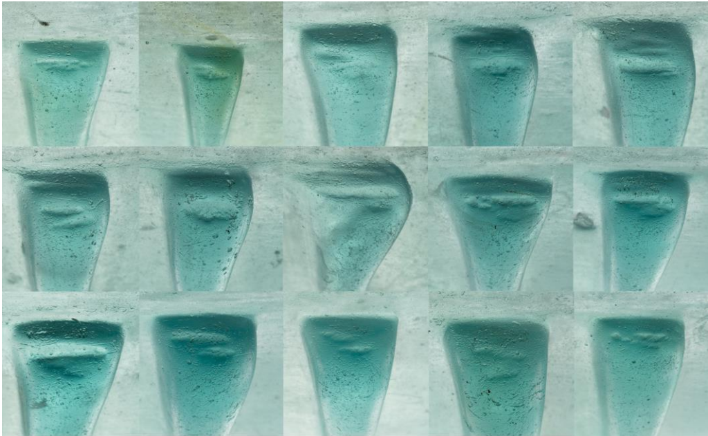
Fig. 20. Ribbed bowl (cat. no. 2): mosaic of detail photos showing in comparison the tooling marks present on the upper part of all the 15 ribs of the vessel.
