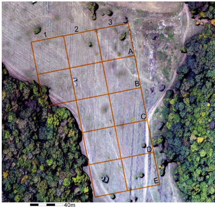
Fig. 13. Celic Dere Monastery/Cassiana site - the geophysical grid overlapped on the orthophotography which was textured on top of the hillshaded terrain model (DSM).
