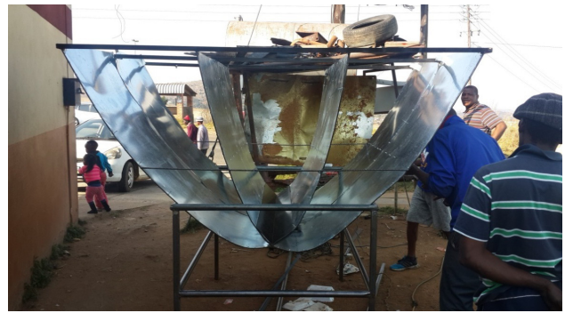
Fig.9. The modified CPC reflector with the frame seater
