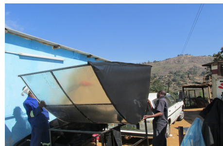
Fig.11. Sides of the reflector covered with polyethylene sheets
