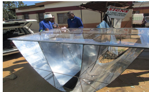
Fig.10. Perspex glass of 4 mm thickness used for the top cover
