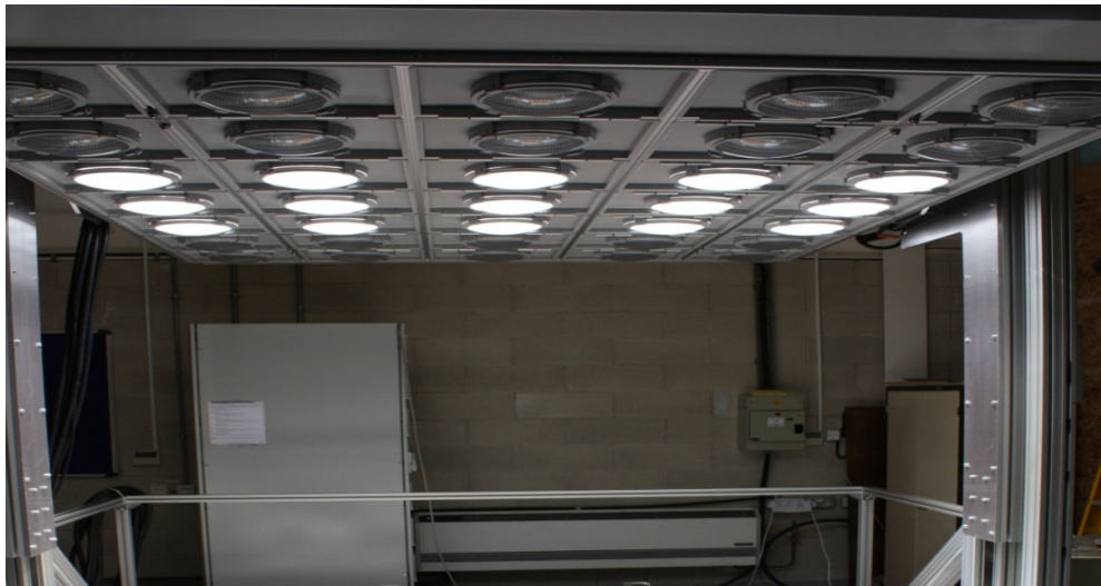
Fig. 1. Solar simulator set-up to illuminate the solar cell at normal incidence angle
