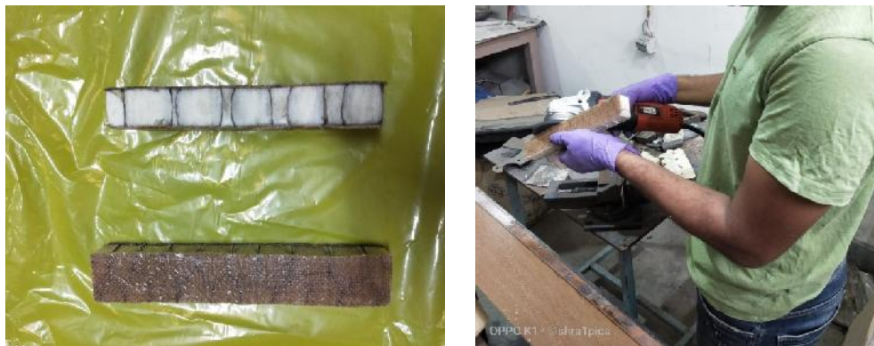
Figure 14: Machining the Component According to the Standards.
