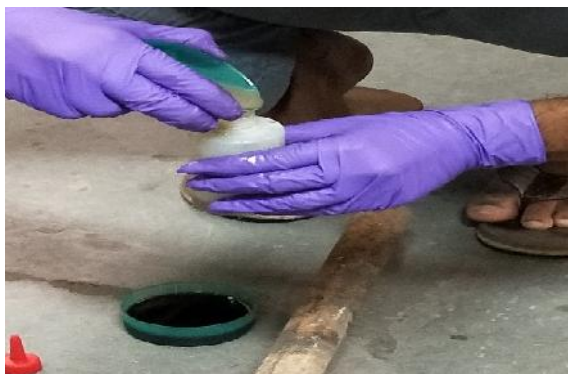
Figure 10: Mixing of Polyol and Isocyanate & Figure 11: Poring of Mixed Liquid Foam.
