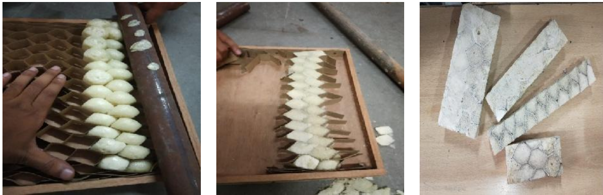
Figure 12: Liquid Foam in Solidifying & Figure 13: Removing of Excess of Foam and Filing .
