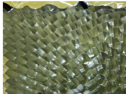
Figure 8: Honeycomb Paper & Figure 9: Honeycomb Aluminum Figure 8 & 9: Spreading of Honeycomb Material.
