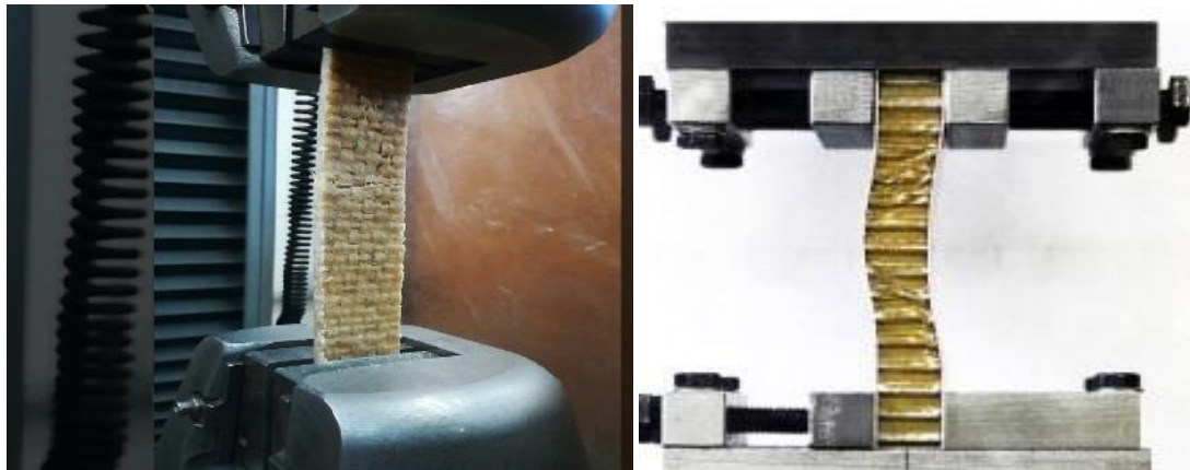
Figure 15: Tensile Test & Figure 16: Compression Test.
