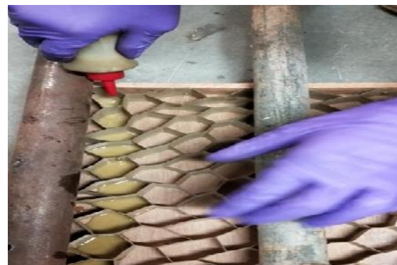
Figure 10: Mixing of Polyol and Isocyanate & Figure 11: Poring of Mixed Liquid Foam.
