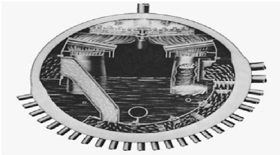
Figure 2: Inside Arrangement of Boiler Drums.
